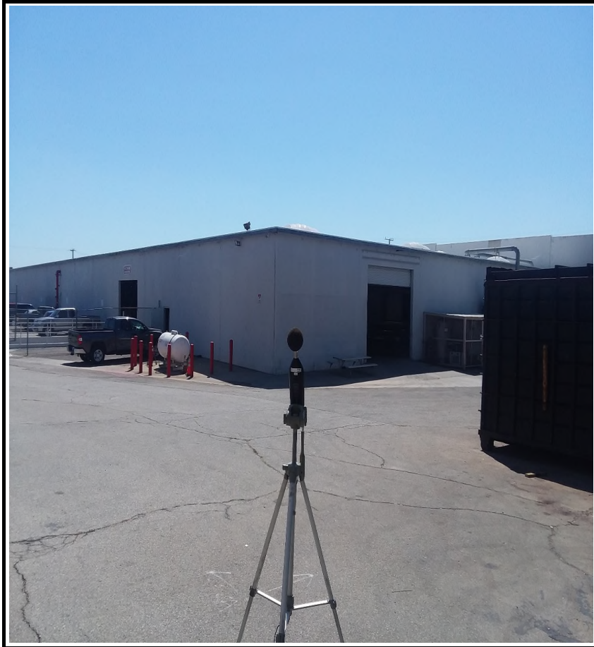
STNM2 looking S towards building 12436 Putnam Street, Whittier. Industrial machinery noise emanating from openings in building.
