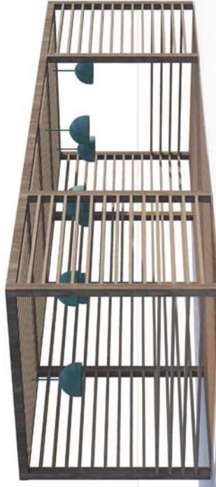
Wood frame and ceiling slats with partial side panel
