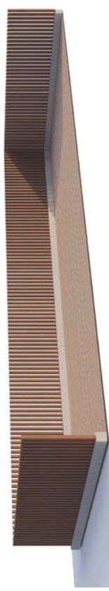
Freestanding metal posts set in concrete curb
