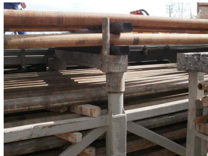
Pads and Boards Between Pipe
